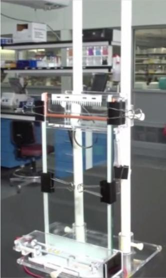
Gel electrophoresis during Sanger sequencing.
