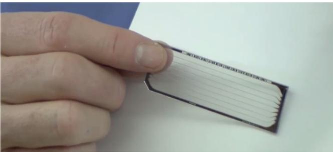
A slide used for Illumina sequencing.
